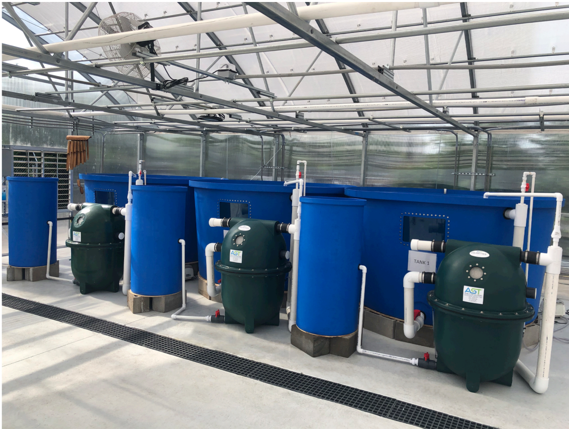
Figure 2 AST's experimental set up of three 4-ton PG6000 systems.
