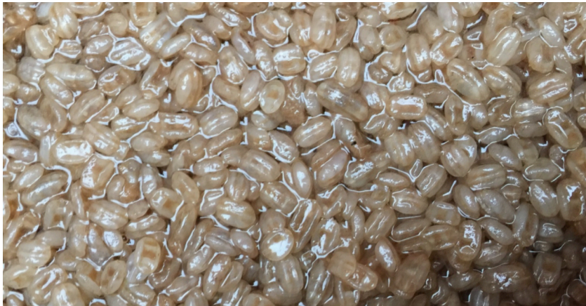
Figure 4 The beads become coated with a nitrifying biofilm. The PolyGeysers® are effective fixed film bioreactors even as they capture solids.
